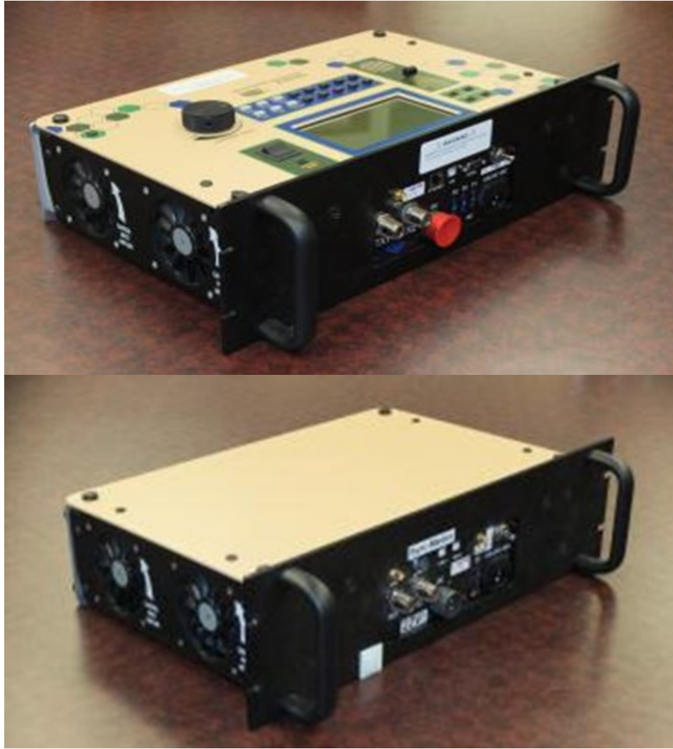
Figure 3.10. Sounder Tx (left) and Rx (right, 1 of 2).
