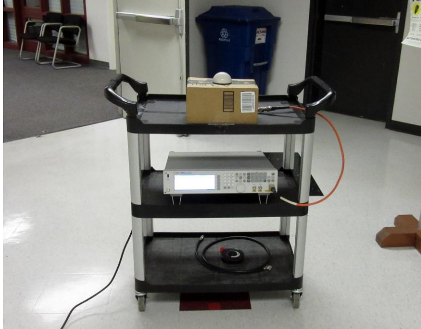
Figure 3.7 Transmitter Antenna set up.
