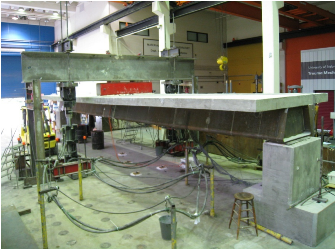
FIGURE 2-18: COMPOSITE TEST SETUP
