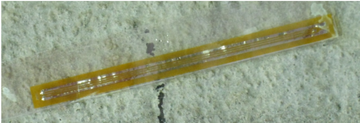
FIGURE 2-15: TYPICAL CONCRETE SURFACE GAGE USED DURING TESTING
