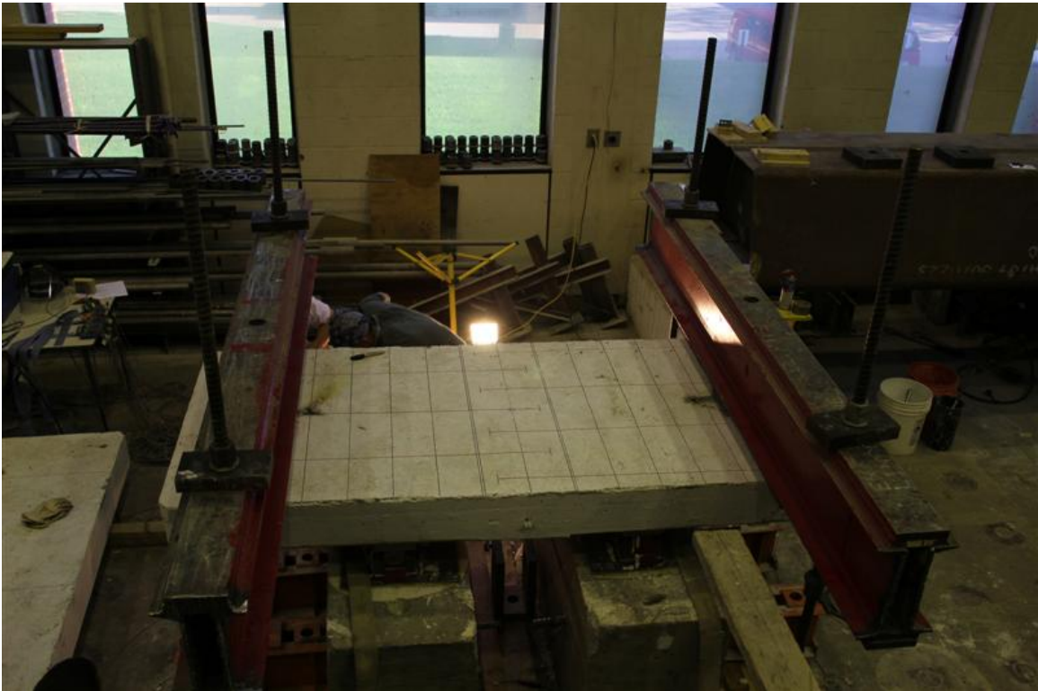
FIGURE 6-11: SLAB TEST SETUP
