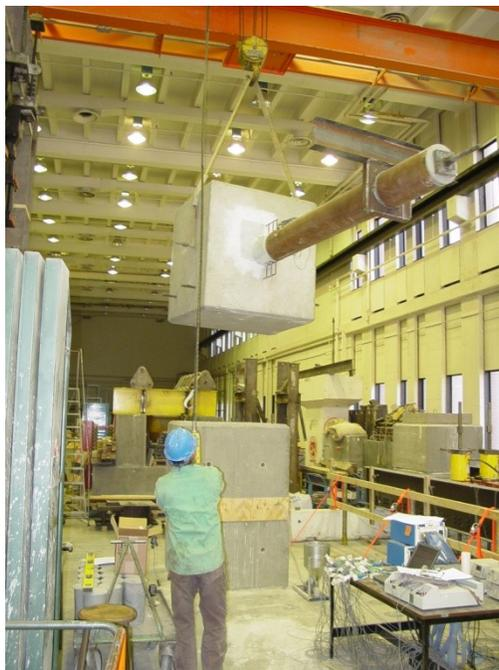
**Figure 4-19- Placing specimen #1 on top of support blocks**
