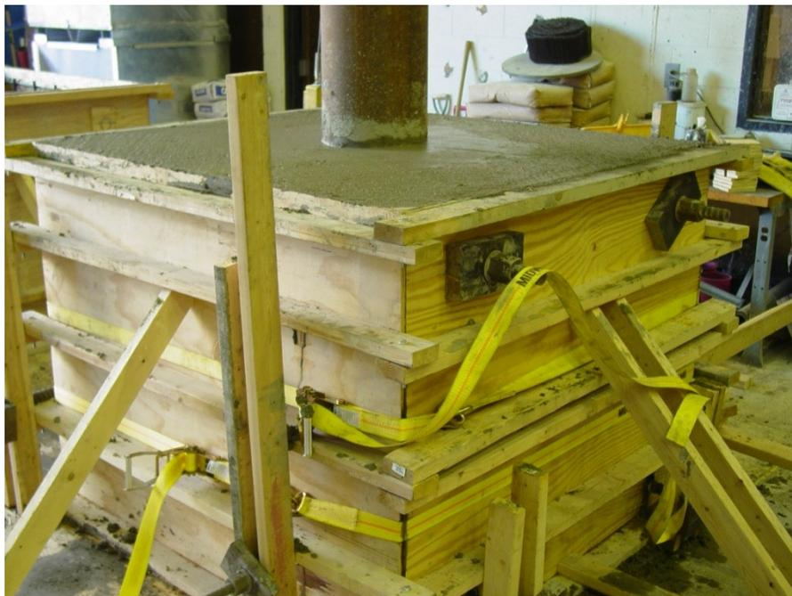
**Figure 4-16- Specimen #1 after the pour**
