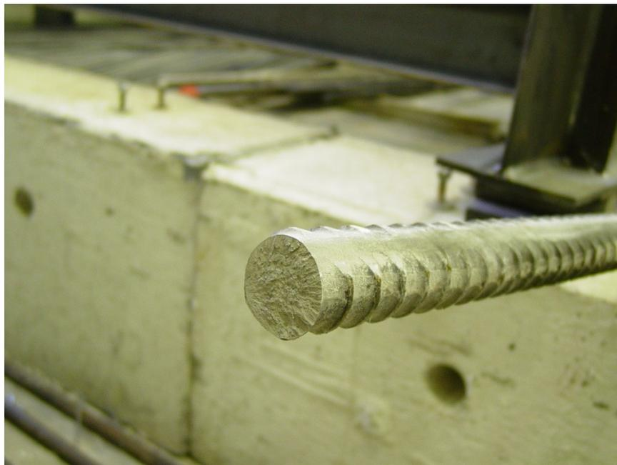
**Figure 4-36- Failure of the dywidag**
