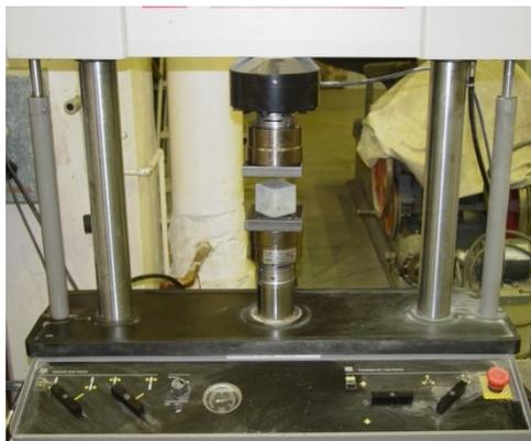
**Figure 4-69- MTS Load frame for cyclic load test**
