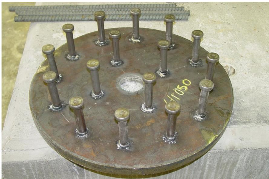
**Figure 4-8- Embedded plate**
