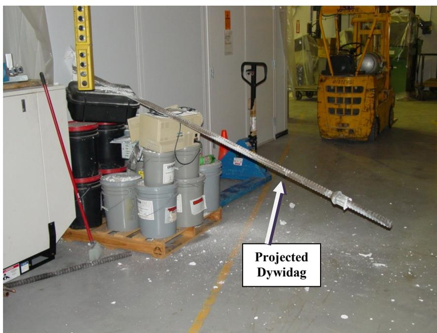
**Figure 4-35- Failure of the dywidag**
