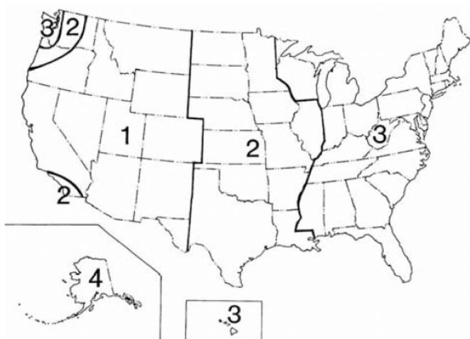
Figure 2-2- Solar Radiation Zones for the United States. (Figure 3.12.3-1 from AASHTO)
