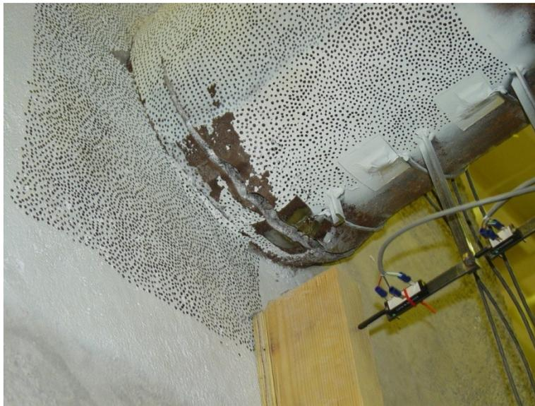
Figure 4-27- Crack completely opened at load stage 3-19 ( $\pm 4.75$  in)
