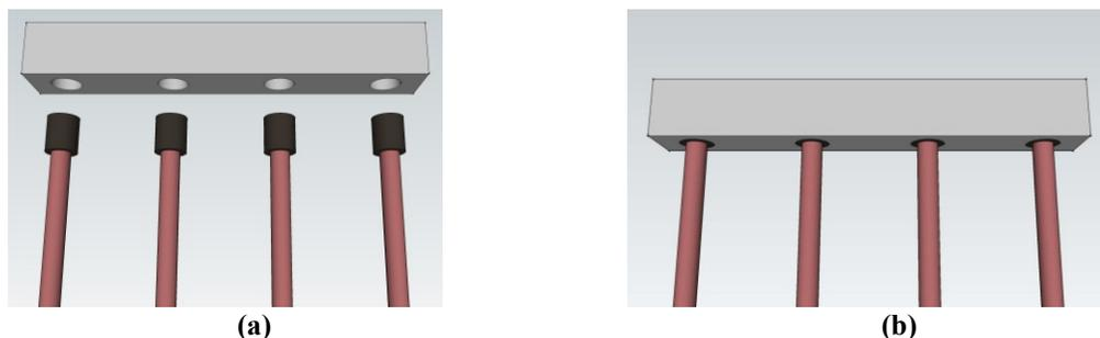
**Figure C41- Prefabricated pile cap**
