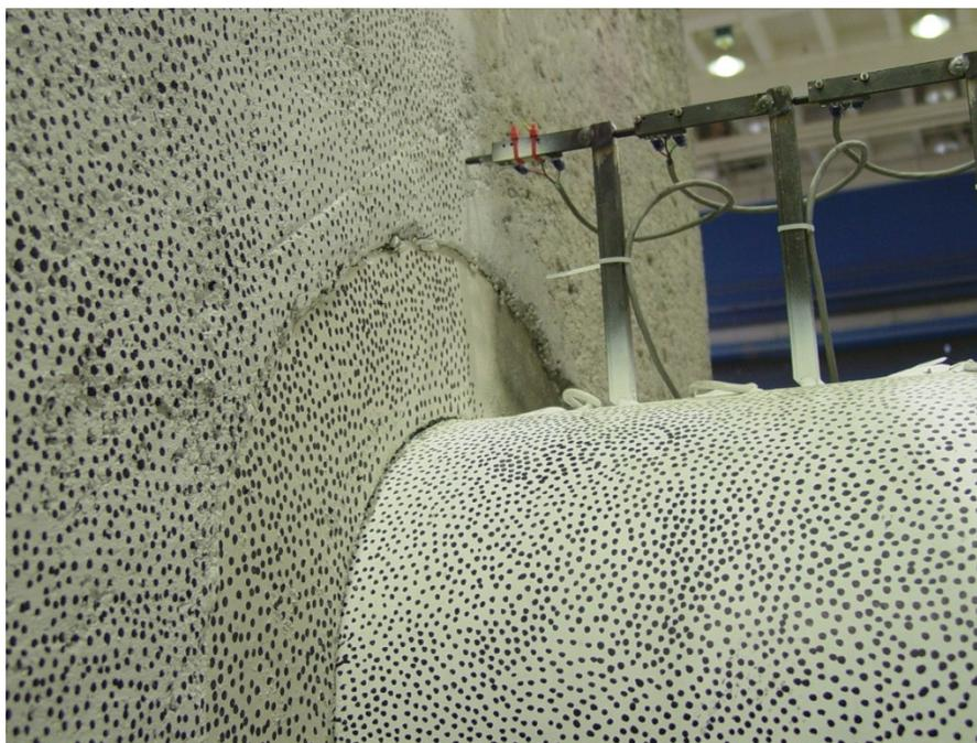
**Figure 4-29- Condition of the connection at stage 1-9 ( $\pm 2.00$  in)**
