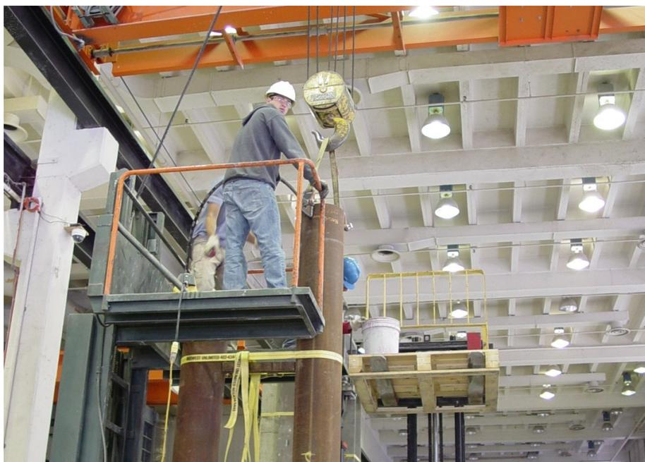
**Figure 4-12- Pouring concrete into the pipe**
