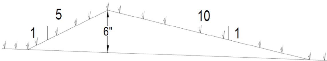
Figure 22: Swale design example check dam profile
