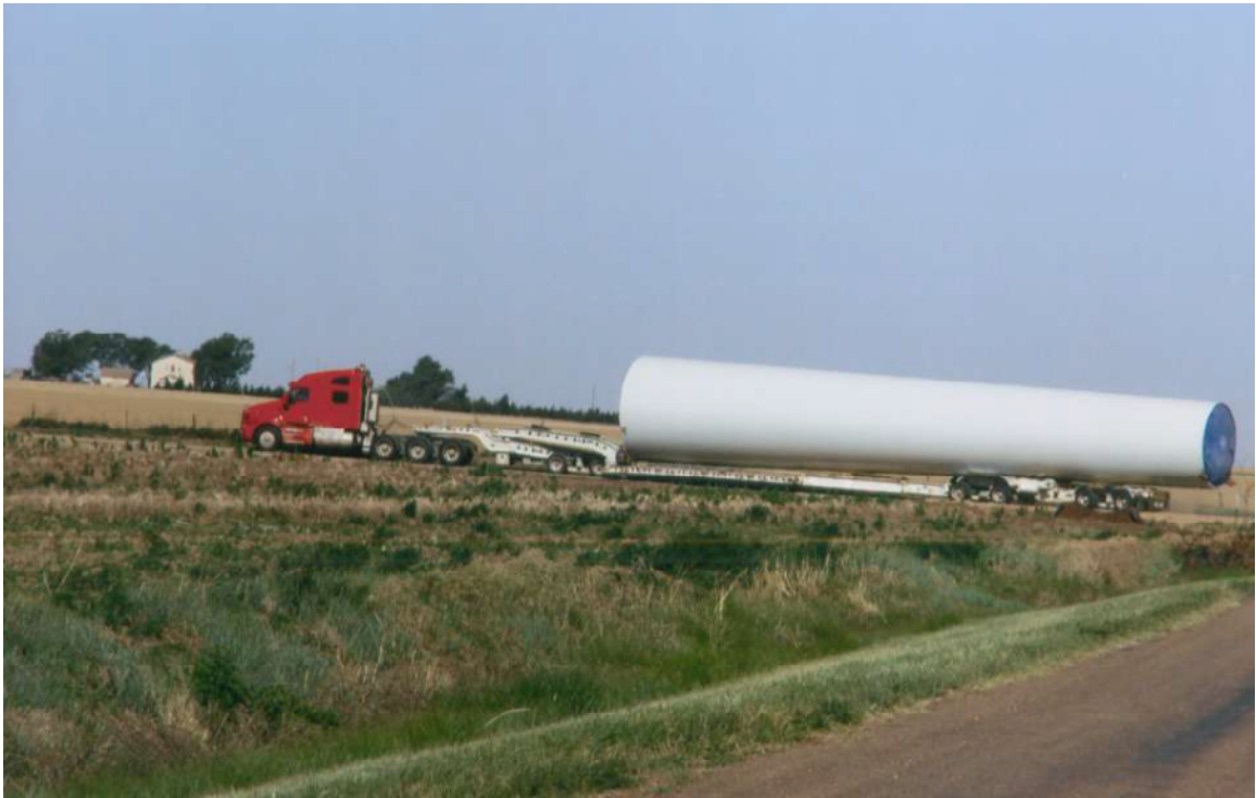
Figure 2-1: Transportation of complete steel tube segments. (Sri, S., 2011)
