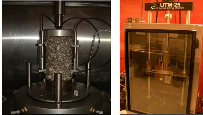
Figure 4-4. A Specimen with LVDTs Mounted in UTM-25kN Testing Station
