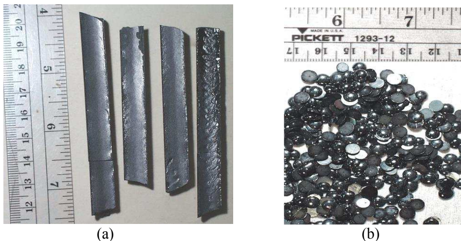
Figure 2.2. (a) Appearance of the ZR Se ingots (~7N) after multi-pass zone purification; the shiny ingot at the extreme left is the purest end while ingot at the extreme right is the impure end. (b) Se dry pellets synthesized from the highly pure ZR ingots.
