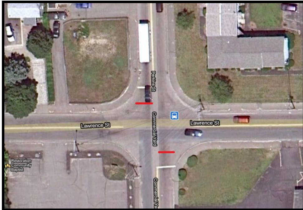
Figure 18. Intersection 74907 Satellite View with Relocated Stop Bars
