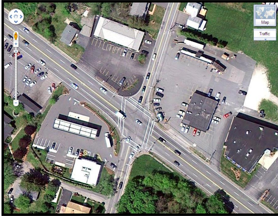
Figure 23. Intersection 348139 Satellite View Showing Skewed Geometry
