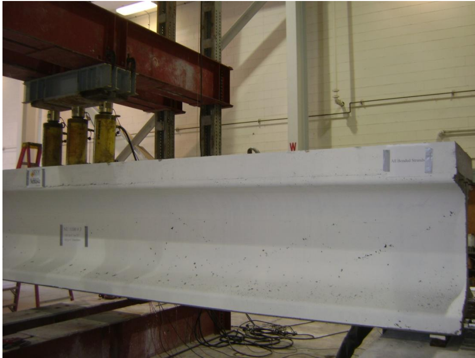
Figure 3.27 NU1100 Development Length Test Setup
