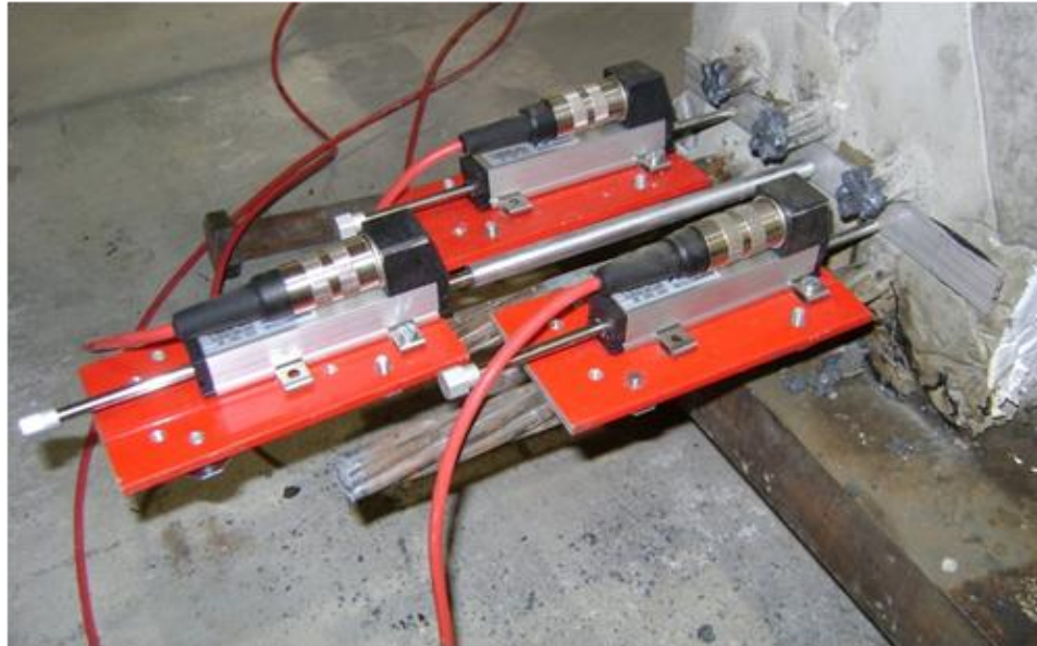
Figure 3.14 Potentiometers Attached to the Bottom Row of Strands
