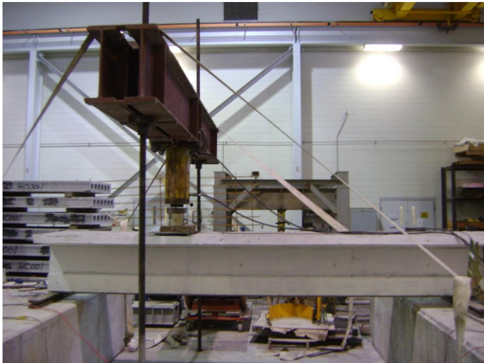
Figure 3.16 T24 Vertical Shear Test Setup
