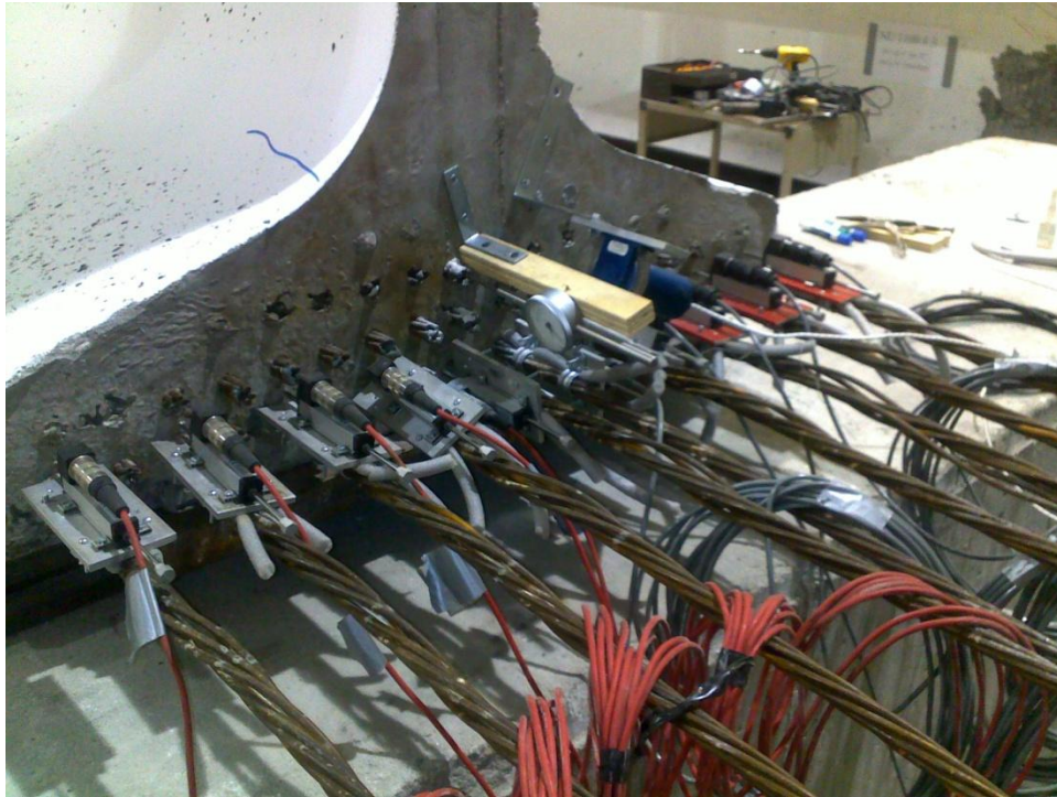
Figure 3.28 Development Length Test Strand Instrumentation
