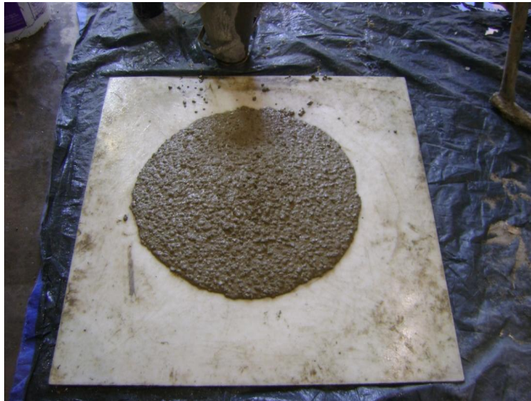
Figure 3.8 T24 Concrete Spread
