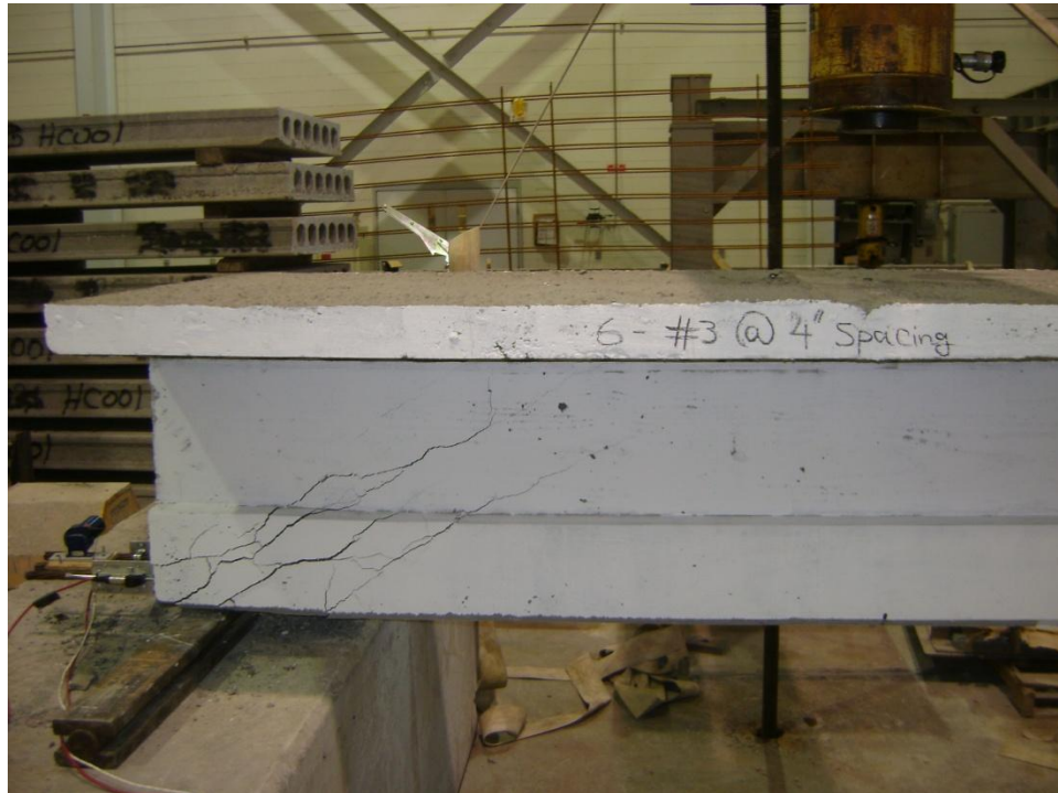
Figure 3.48 T24 T-4-1.0h-D Post Shear Test
