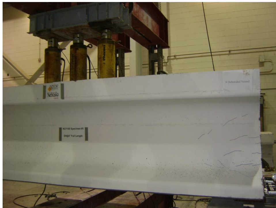
Figure 3.30 NU1100 Vertical Shear Test Setup
