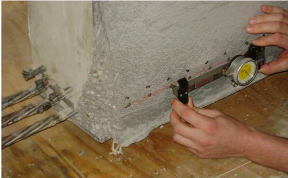
Figure 3.11 Measuring Strain in Concrete for Transfer Length Estimation
