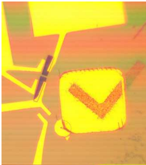
Figure 4.3 Optical image showing trench patterns after exposure and the rest of the sample being covered with PMMA.
