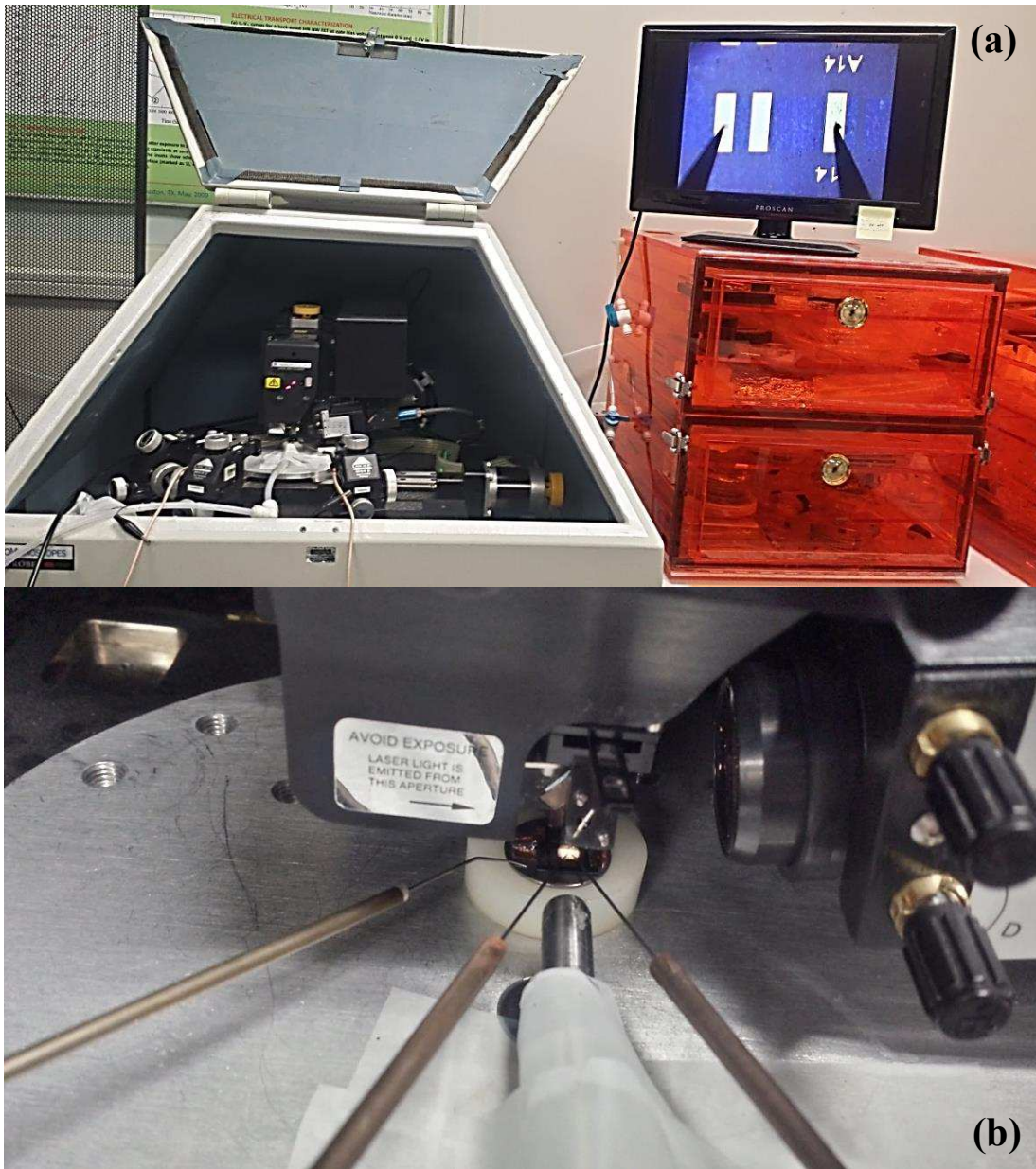
Figure 7.6 Graphene/InN NW heterojunction sensing setup (a) showing how the probes are placed on the sample and (b) showing a close-up of the device.
