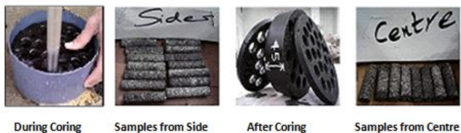
Figure 4.4 Torsional Bars Extraction SGC Fine Aggregate Matrix
