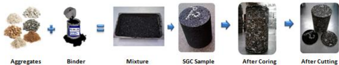
Figure 3.1 Sample Fabrication of Asphalt Concrete Mixtures
