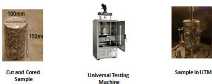
Figure 3.3 Installing the Asphalt Concrete Samples for Tests
