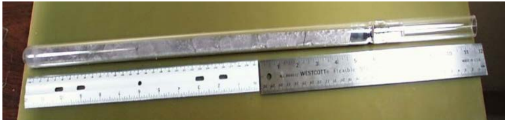
Figure 3.2. Zone refined (ZR) Cd ingot within a quartz ampoule; pure precursor material is on the right side while segregated impurities are on the left side of the ampoule.
