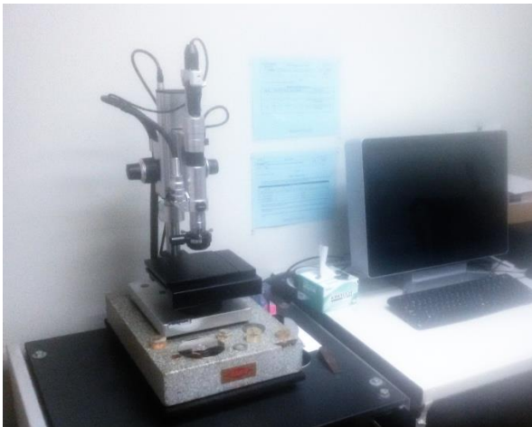
Figure 3.8 Hirox KH-8700 3D DIGITAL MICROSCOPE
