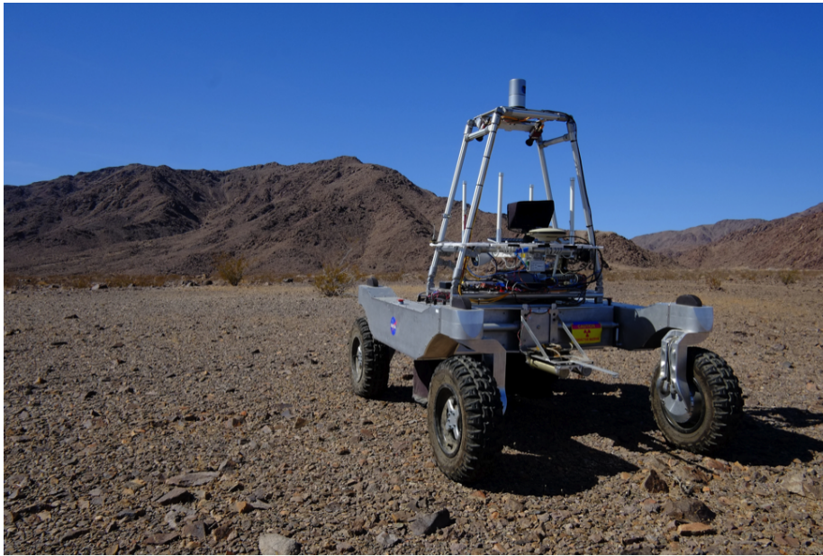
Figure 4.1: KReX2 in the Mojave desert. The stainless steel and cadmium cylinders of the Neutron Spectrometer are visible on the rear of the vehicle.
