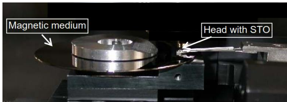
Fig. 1.11. Experiment setup of MAMR using STO [18].
