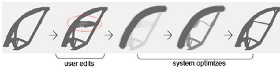
Figure 5.9: Users can suggestively add material to a generated result (circled strokes), which prompts the system to re-run the optimization and attempt to add structures accordingly.
