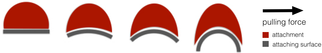
Figure 3.13: To test strapping in print-to-affix, we increased the curvature between the attachment and the attaching surface and exerted tangential pulling force.
