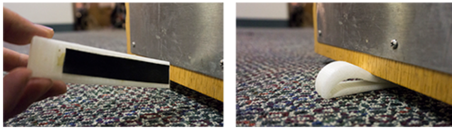
Figure 6.7: Embedding a piece rubber to make a functional door stop.
