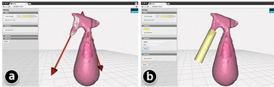
Figure 4.8: To specify clatching, the user selects the two parts of the object that are being clutched and then the fulcrum. The red arrows indicate the directions of the clutching arms (a). The user can generate a lever for clutching the spray bottle, while holding its body in hand (b).
