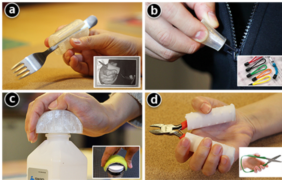
Figure 4.17: Replicated wrapper/extension examples. Ninjaflex was used for the fork wrapper (a), zipper handle extension (b), and the bottle lid wrapper (c). Nylon-based soft material was used for the cutter.
