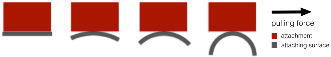
Figure 3.10: To test print-over in comparison to printing in one piece, we used both techniques to print attachments on surfaces with varied curvatures and then exerting tangential pulling force.
