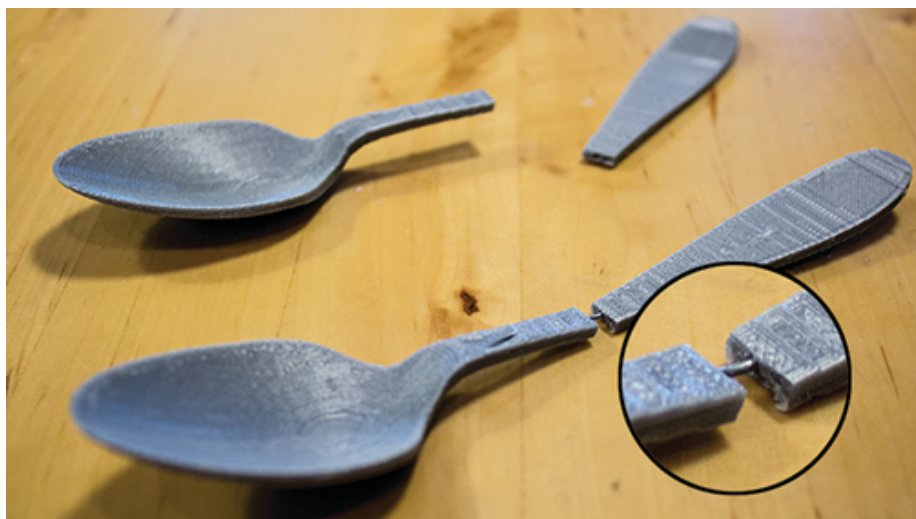
Figure 6.8: Embedding wire straightened from a paper clip into a spoon avoids snapping, which could be dangerous to the user during breakage.
