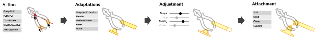
Figure 4.4: The design workflow of Reprise. Start with specifying the types of action applied on an object, which serves as input for generating user-selected adaptations . The initial design can be further customized by adjusting a set of parameters. Finally, extra fasteners can be added to make adaptations more attachable onto the object.
