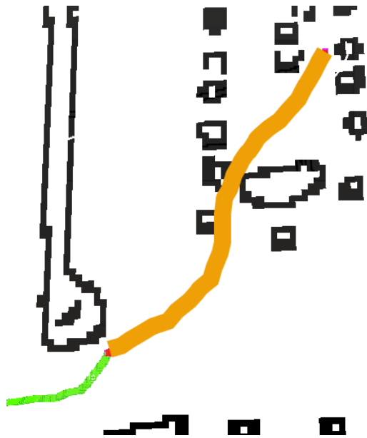
Figure 6.16: An example of the EXECUTEMOTIONPRIMITIVE controller moving down to the left. The thick sections in the center do not have an adequate wall or landmark near by, so the planner uses several of the standard motion primitives to avoid the obstacles. Note: the line is drawn thicker than the robot footprint for clarity; the robot trajectory remains collision free.
