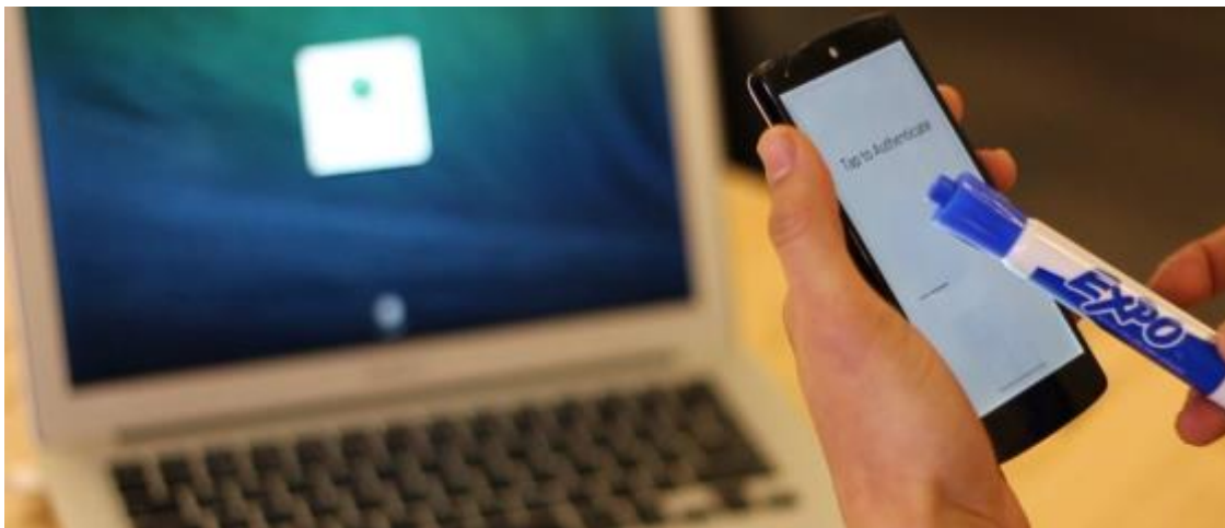
Figure 10. With Thumprint, groups of users learn a single, shared secret knock that they enter on a surface instrumented with (or containing) an accelerometer and microphone (here, a smartphone) in order to authenticate.
