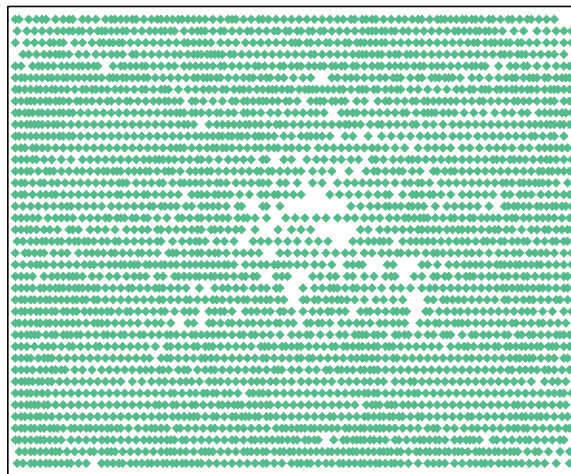
Figure 5.1: Gate placement created by a commercial place-and-route tool for benchmark circuit c7552 [23].
