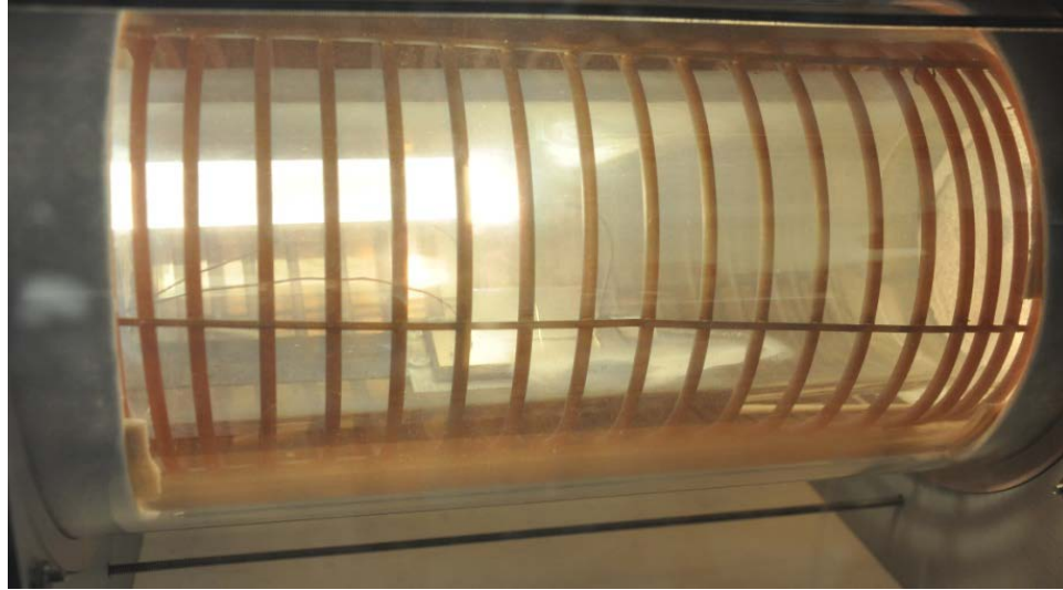
Figure 2-12 Hot Zone of the CAB Furnace
