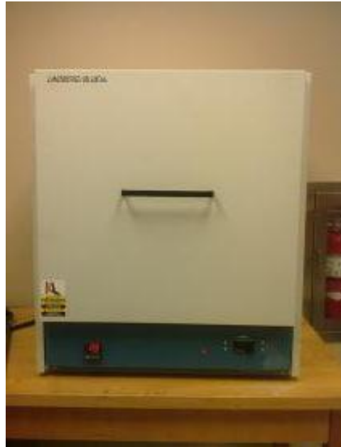
Figure 3.1 Lindberg/Blue M BF5114841 box furnace.
