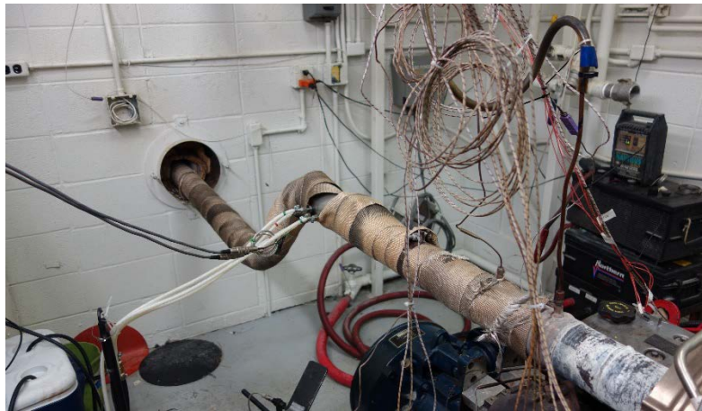
Figure 3.3 Exhaust pipe with pressure transducers installed.
