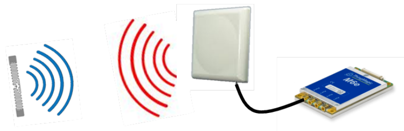
Figure 2.1: Major components of a passive RFID system
