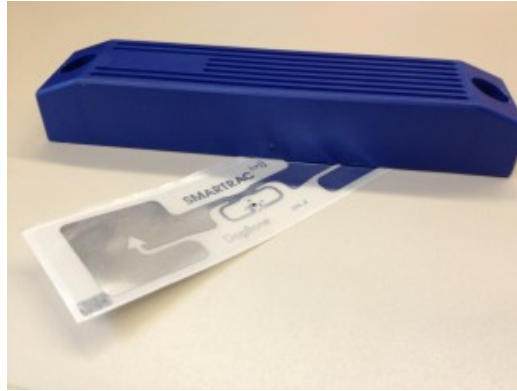
Figure 2.2: Passive RFID tag and active RFID tag (atlasRFIDstore)
