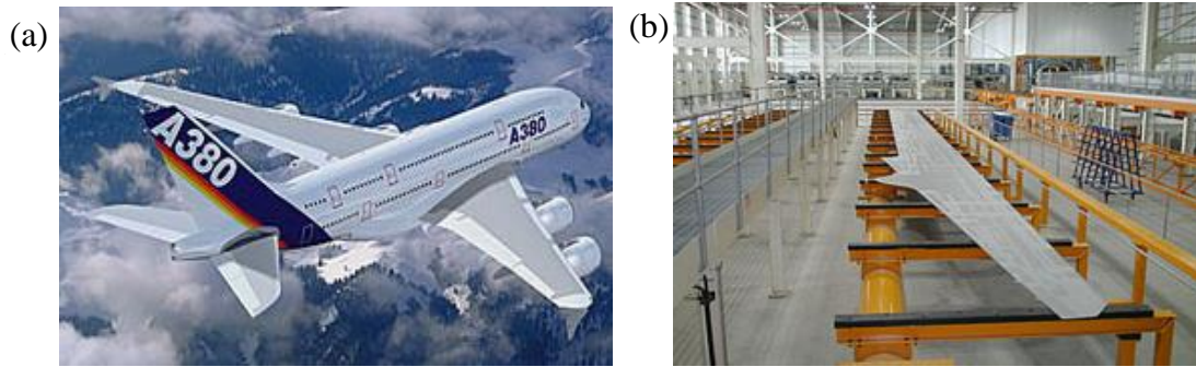
Figure 2.1: (a) Airbus A380 in flight; and (b) View of the internal face of a starboard wing skin panel made of Al 7050-T7451 alloy (Atkins Ltd, 2012).
