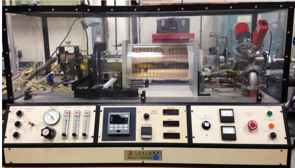
Fig. 2.10 Transparent high temperature CAB laboratory furnace system
