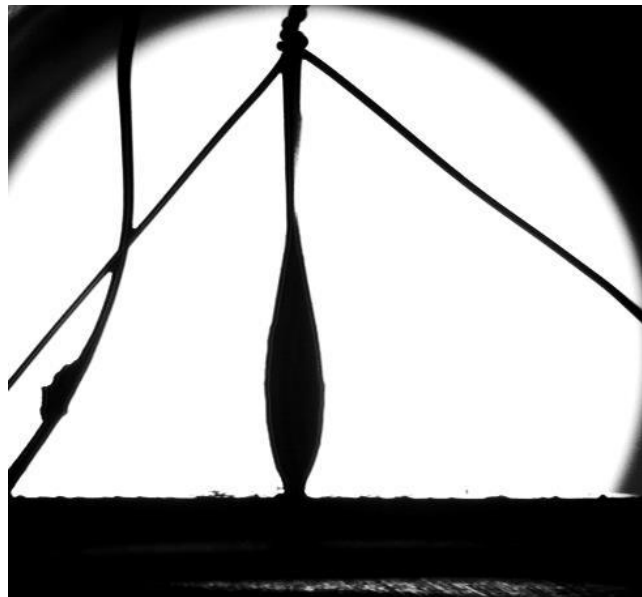
Fig. 6.17 Molten clad metal spreading on vertical AA3003 plate with non-wetting horizontal surface (Experiment 05052015)
