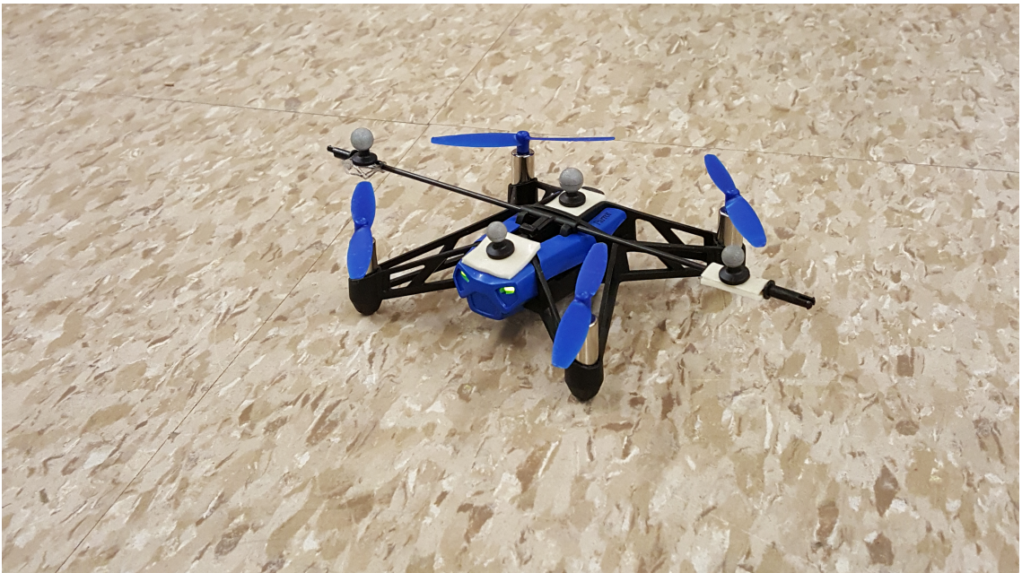
Figure 4.3: A picture of the Rolling Spider quadcopter with 4 attached markers for motion capture. The markers are arranged in a planar diamond configuration.
