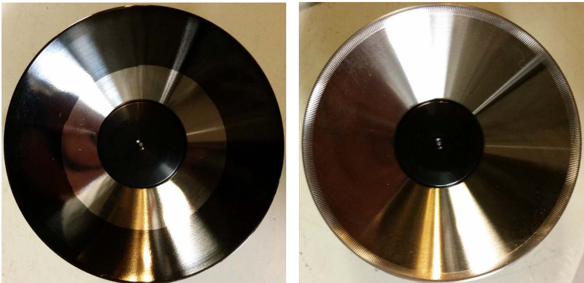
Figure 2.1. Unserrated (left) and serrated (right) 65mm bell-cups.
