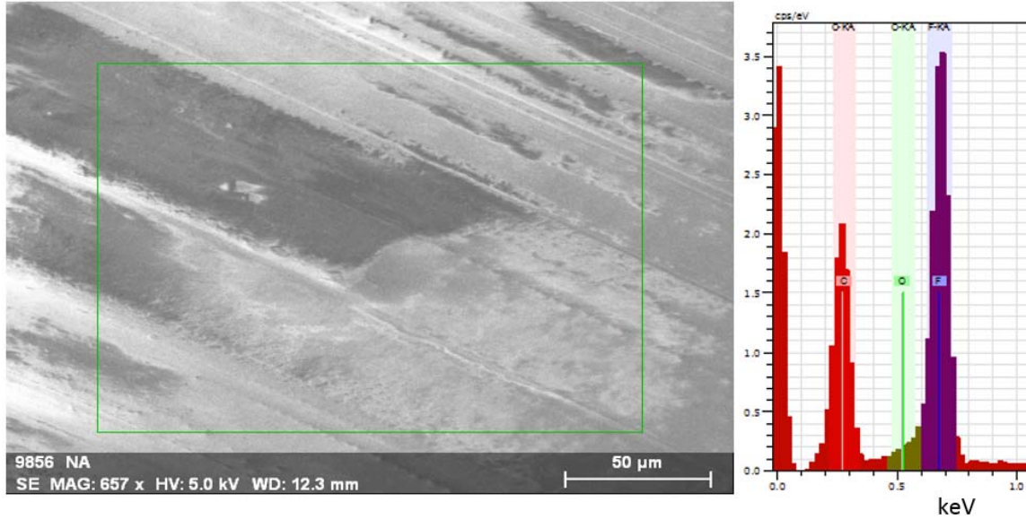
Figure 4.18: SEM image with EDS analysis of the stationary PTFE seal surface. (Seal 7)
