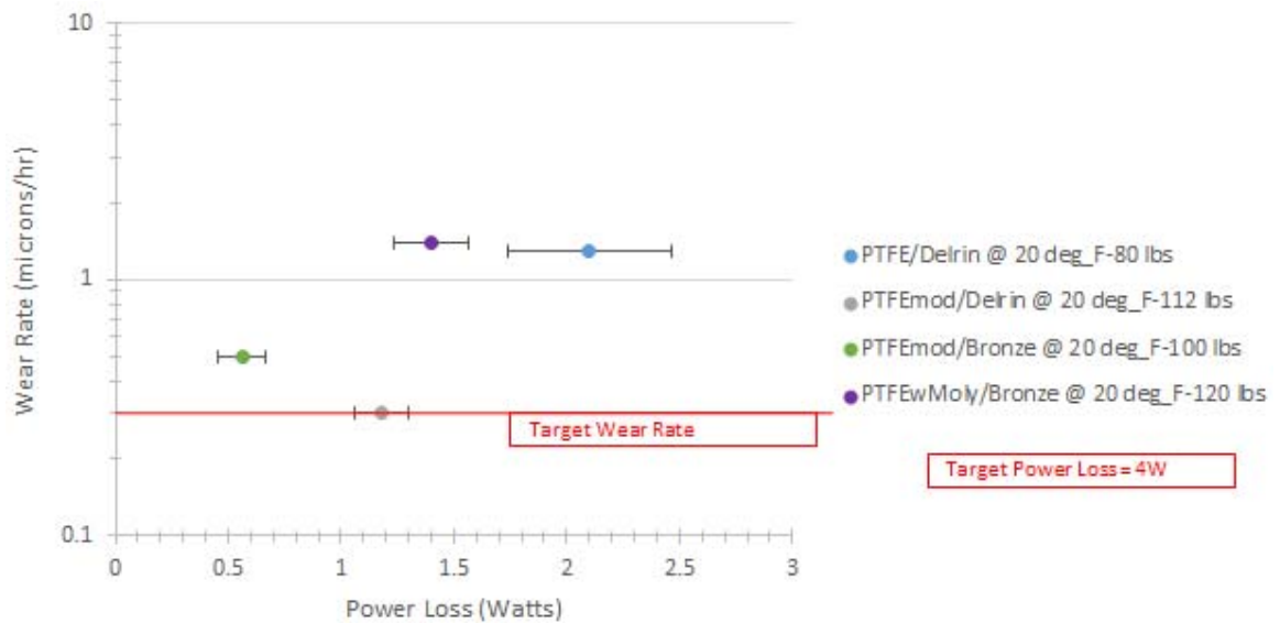
Figure 4.11: Wear rate and power loss results of low temperature testing with face load
