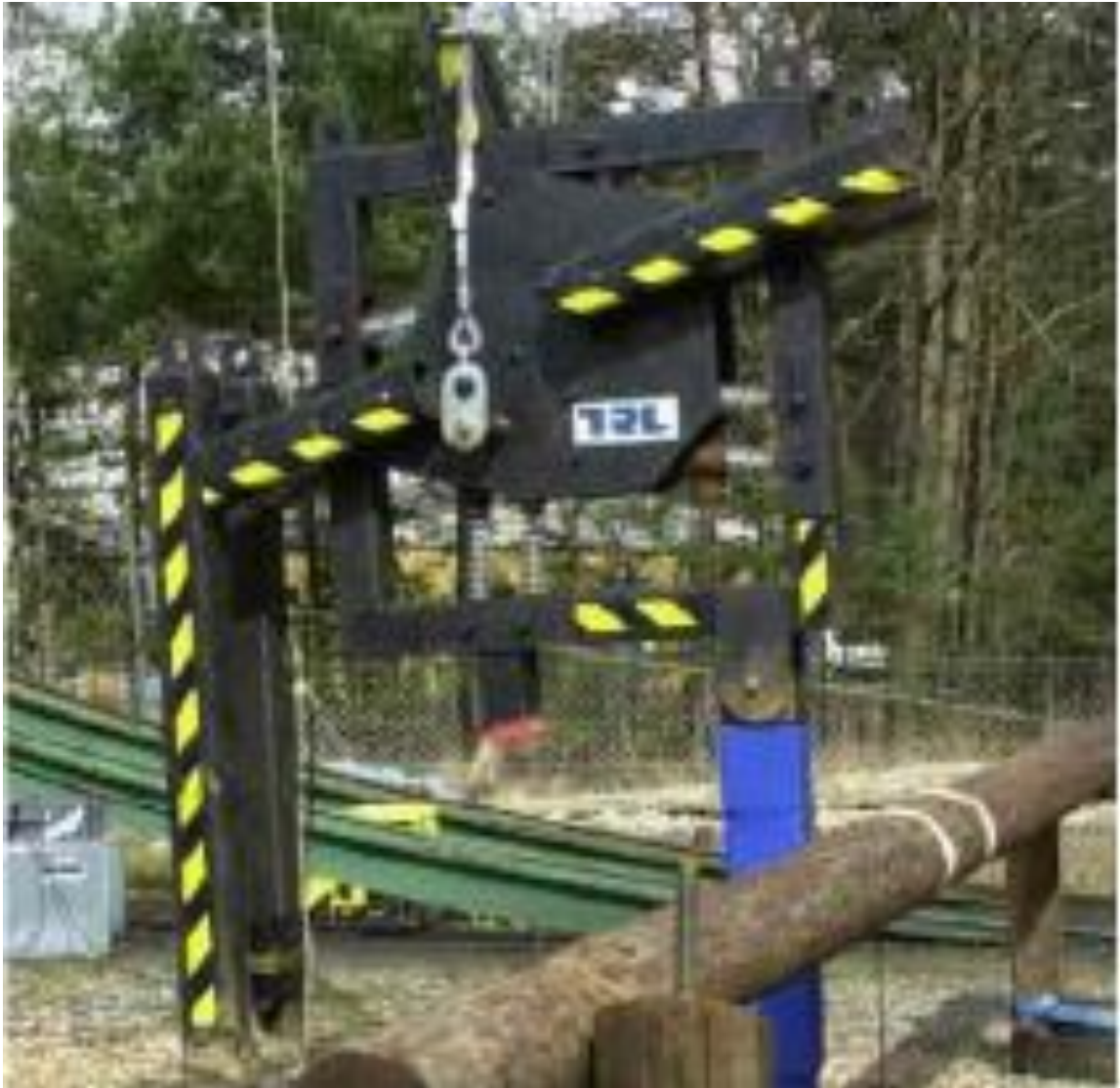
Figure 2.1 Image of NED, a horse simulator impact tester created by TRL [1]
