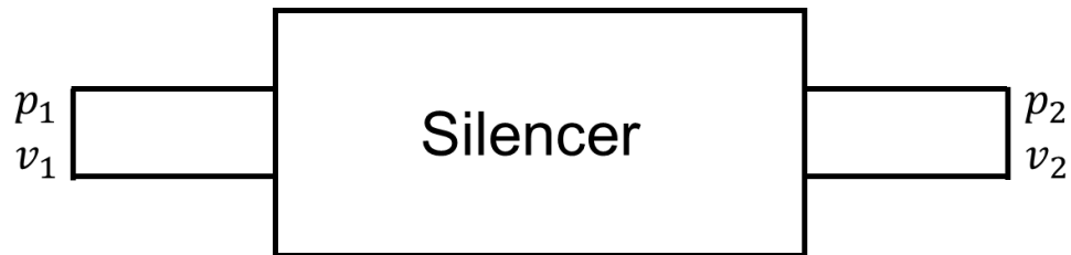
Figure 1.6 Four-pole method for TL calculation.
