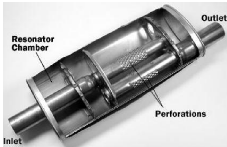
Figure 1.2 Typical reactive silencer. (Potente, 2005)
