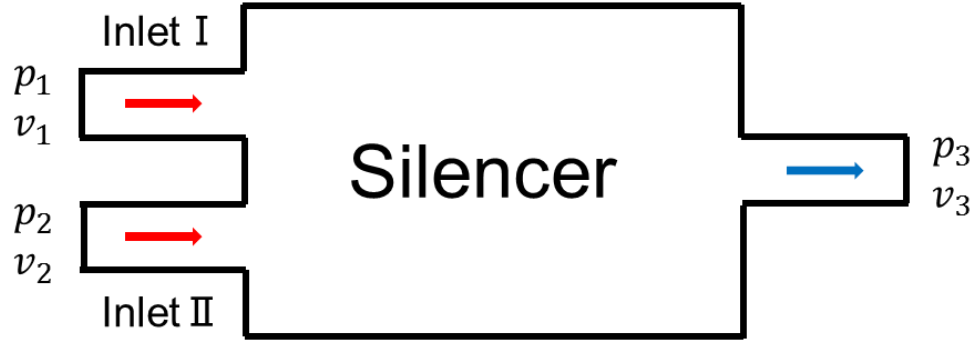
Figure 3.1 Two-inlet and one-outlet silencer.
