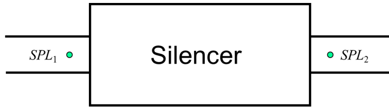
Figure 1.5 Definition of noise reduction of a silencer.
