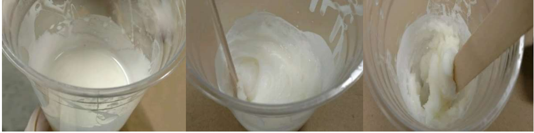
Figure 18: Progression of Aero-Epoxy Viscosity a.) Less Than 1:1 b.) Between 1:1 and 1:2 c.) 1:2 and Greater
