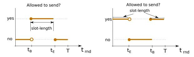
Figure 4.2: Defining a TDMA slot and respective boundaries. Left) Boundary  $t_B$  is less than  $t_E$ . Right) Boundary  $t_B$  is greater than  $t_E$ . Inside a slot, a node is allowed to transmit packets (cf. Equation 4.2). Slot length is also depicted (cf. Equation 4.3).
