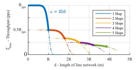
Figure 3.4: Maximum network throughput as function of distance –  $\zeta_{\max}(d)$ , in packets per second. Each colour represents a different number of hops in use in the network, described by a different section of Equation 3.17. Number of hops  $h \in [1, ..., 5]$ , and updated at certain distances given by Equation 3.18. Link PDR assumes  $\alpha = 10.6$ .
