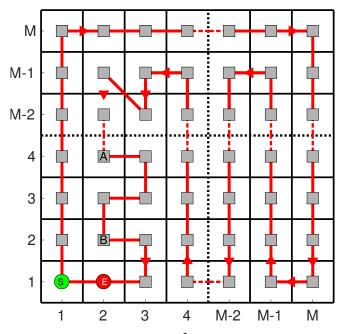
Figure 7.5: Square AoI with odd number of cells ( $M^2$ ) to visit. Side size is W. Red path describes the shortest tour, and it starts at "S", it ends in "E", and restarts at "S" again. It includes one diagonal edge, so tour length  $d \approx d_{\min}$ .
