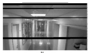
Figure 6.11: Video stream snapshot with relay positioned at: a) midpoint between source and sink, showing plenty of packet losses (black lines); and b) 0.6 of the distance between source and sink (x = 13m), leading to balanced links and fewer packet losses.
