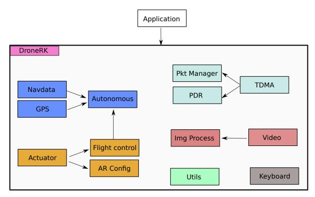
Figure 8.1: Drone-RK software is comprised of several modules, spanning from actuation and sensing to communications.
