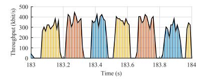
Figure 3.5: Typical packet traces on a line network with three hops. End-to-end a rate is  $\approx 90 \text{kB/s}$ . Each colour identifies packets sent from a different UAV. Round is 450ms long, and transmission slot is 100ms. These packet traces were captured by a monitor node, using Wireshark (2016).
