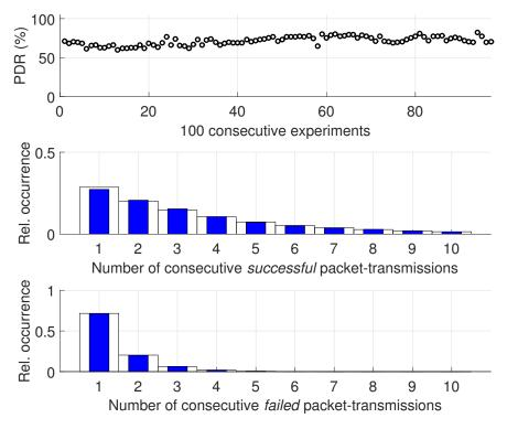
Figure 3.2: Top figure shows typical PDR values of multiple consecutive experiments performed over time, under a given condition of orientation, distance and packet size. Its variation and relative occurrence of consecutive successful/failed packets (colored bars) follows the same trend as a pure Bernoulli experiment (white bars). These plots correspond to the probability mass function (pmf) of geometric random variables.
