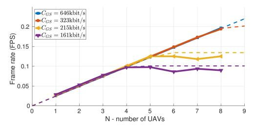
Figure 7.6: Maximum global frame rate versus number of UAVs sweeping the AoI, under different channel bandwidths. AoI: L = 20m, M = 4.
