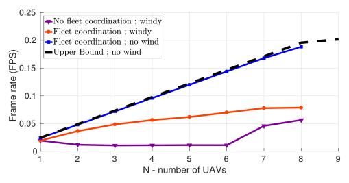
Figure 7.8: Maximum global frame rate to sweep the AoI, with wind gusts pointing north at 6m/s with and without our formation algorithm in place. AoI: L = 20m, M = 4,  $C_{GS} = 323$ kbit/s
