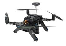
Figure 1.4: Intel Aero research platform comes with a vast set of external sensors.
