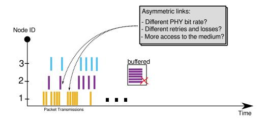
Figure 5.2: Inefficiencies such as buffered packets and wasted bandwidth are created when all nodes are allowed to transmit concurrently and asynchronously, and links have different characteristics such a PHY rate or packet loss. The source, node 1, is transmitting faster than node 2 can cope with.
