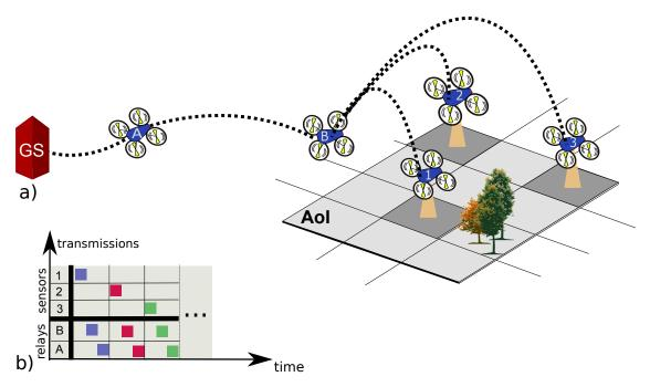
Figure 7.3: The network model encompasses: a) a multi-hop backbone of relay-UAVs that connects the sensor-UAVs (in the AoI)t to the GS; b) a TDMA network access scheme that grants one slot to each sensor-UAV for its exclusive use.
