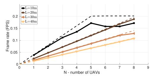
Figure 7.7: Maximum global frame rate versus number of UAVs sweeping the AoI, with different cell sizes L.  $C_{GS} = 323$ kbit/s. AoI: M = 4.
