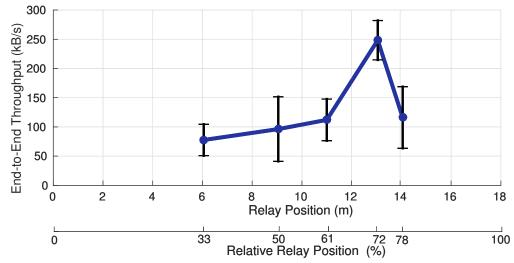
Figure 6.12: Measured end-to-end throughput. Placing the relay at midpoint (x=9m) is not optimal, again. At x=13m, throughput is three times higher.
