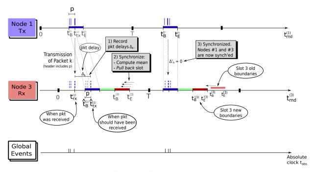
Figure 4.4: Illustration of TDMA self-synchronization mechanism taking place.
