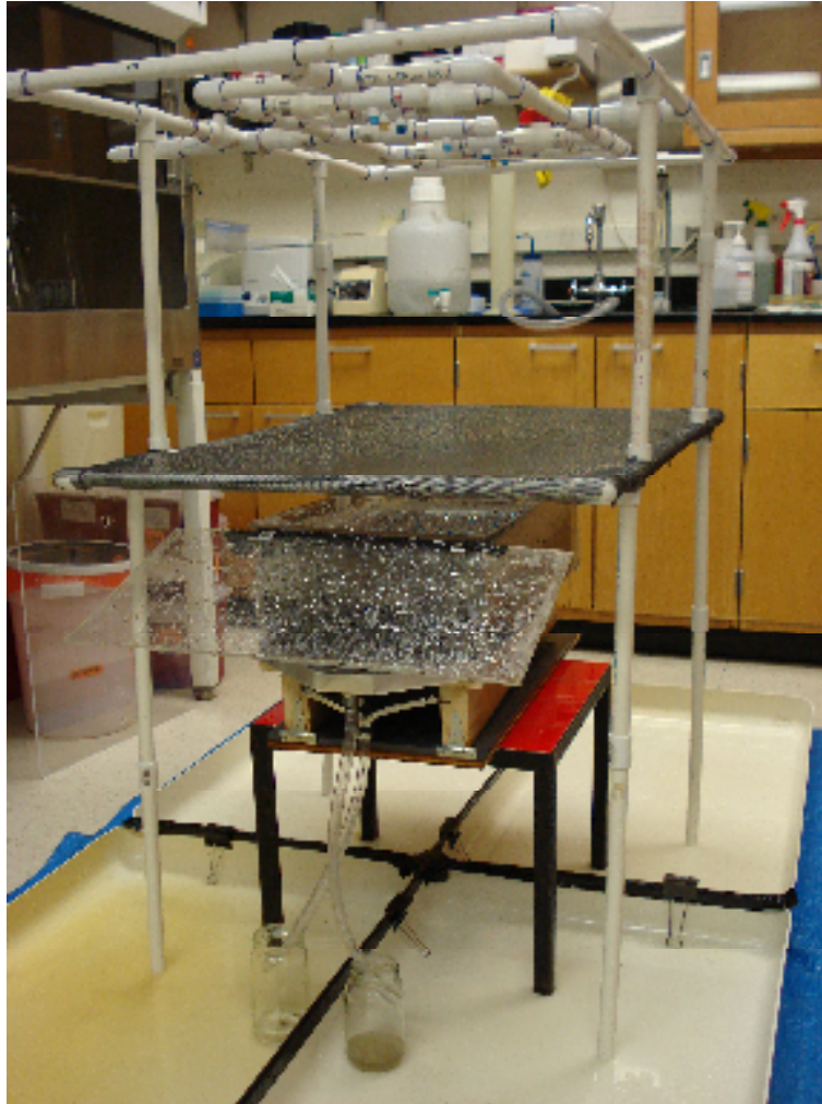
Figure 4.9. Complete laboratory-scale rainfall simulator and tilting soil bed system.
