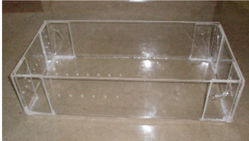
Figure 4.4. Completed soil box with holes for surface and near-surface runoff collection.
