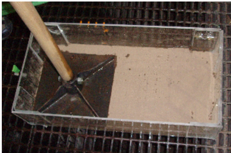
Figure 4.6. Preparation of soil beds. The soil beds were packed in one-inch layers, tamping and adding water to each layer to provide compaction similar to natural field conditions. After the addition of all three layers, the beds were watered regularly to bring the soil back to natural moisture conditions and approach natural compaction.
