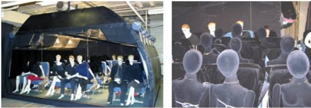
(a) Front view of the aircraft cabin. (b) Manikins and seats covered by black fabric
