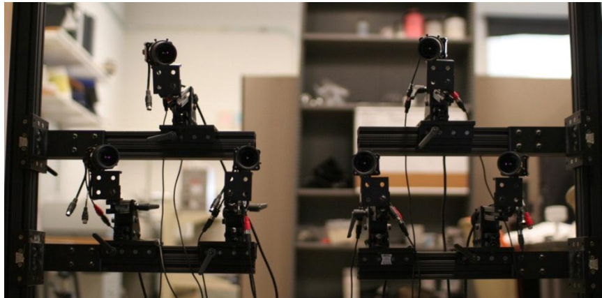
Figure 24: Motion capture camera system used for real-time LPT prototype development
