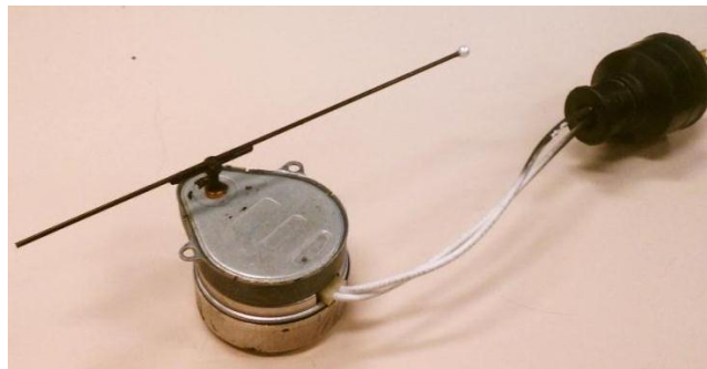
Figure 45: Test object to provide constant tangential velocity to a 3mm white bead
