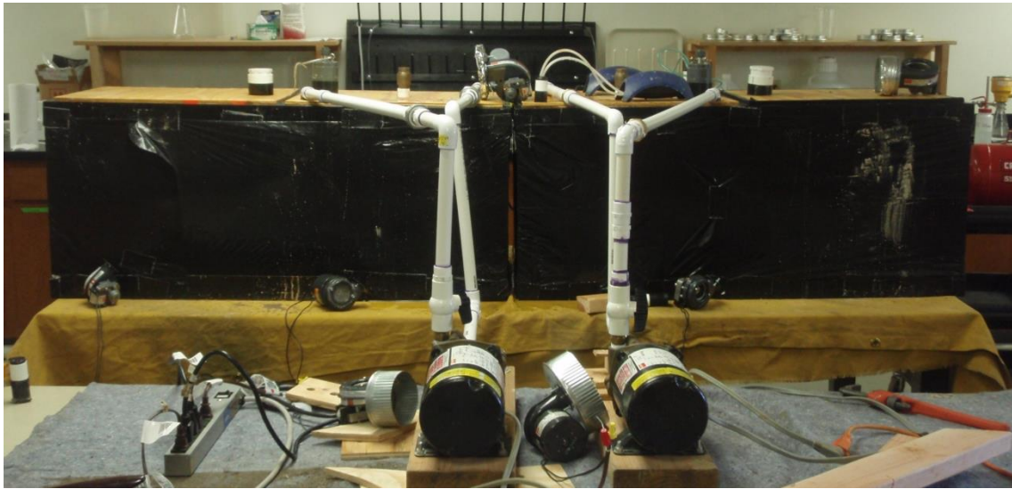
Figure 2. Photograph of the two treatment tanks. Pumps and fans can be seen in the foreground. Aeration pumps (blue) can be seen resting on top of the tank on the right.
