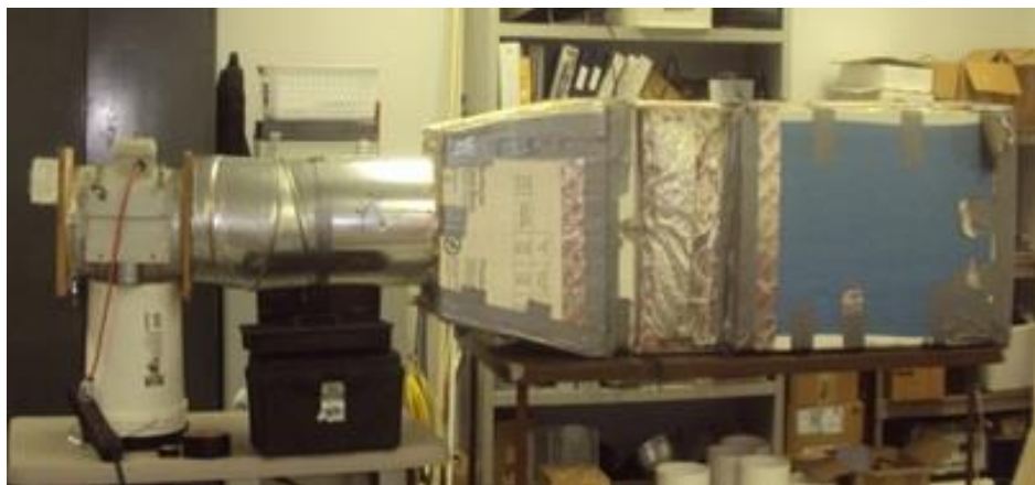
Figure 3.7: Wind tunnel arrangement used in the experiment.
