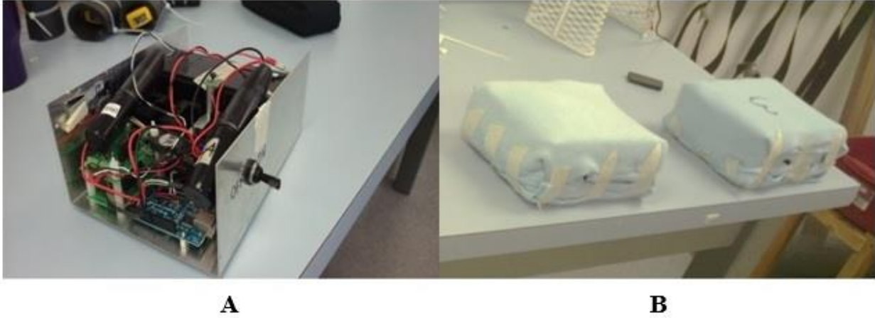
Figure 3.5: Electronic chicken (A) without wrapping (B) with a double layer of fleece fabric wrapping.
