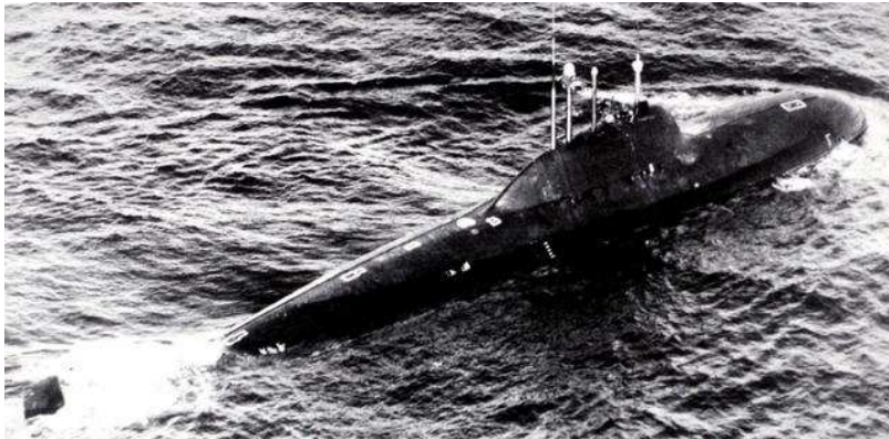
Figure 0.3 Russian Alpha-class submarine with double Ti-based superalloy hull. It is the first submarine whose whole shell is made of Ti-based superalloy. ( http://en.wikipedia.org/wiki/File:Alfa_class_submarine_2.jpg )
