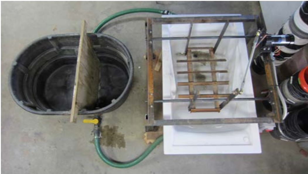
Figure 4.5: The final root washer design meeting all necessary criteria
