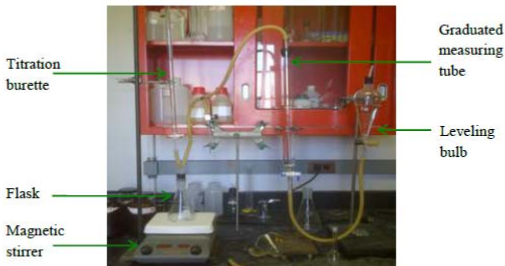
Figure 3.3. A photograph of a chittick apparatus used for CO 2 loading measurement.
