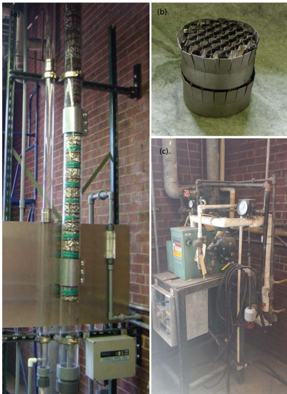
Figure 3.2. Photographs of the bench scale, packed bed absorption column setup: (a) the packed column; (b) a packing unit (10 cm diameter by 10 cm high) (c) Chromalox steam generator.
