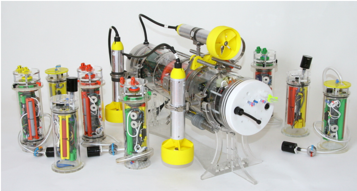
Figure 3.1: Depth adjustment system with AQUANODE and underwater robot AMOUR [19].
