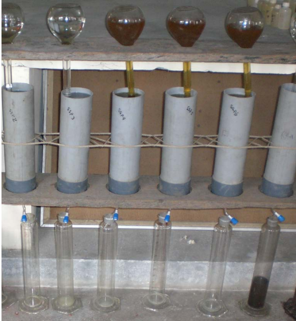
Figure 8. Constant-head flask arrangement designed for our experiment by Dr. Khajanchi Lal.
