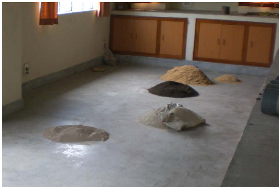
Figure 4. Sorbents prepared for column packing. Note (from back right): ground rice husk, sawdust, sugarcane bagasse, and gypsum. Powdered activated carbon not pictured as it is packaged commercially.
