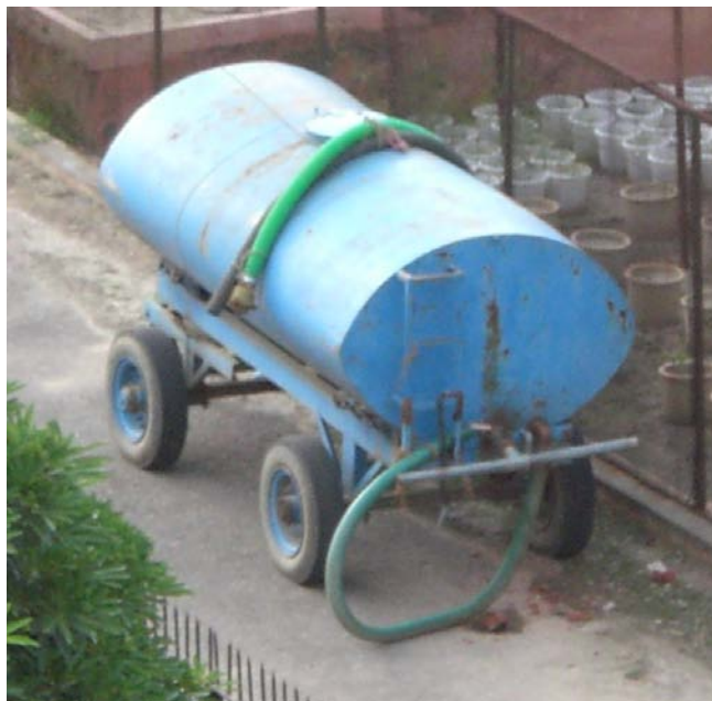
Figure 5. Steel storage tank for native wastewater collected from the wastewater stream near Site 1.
