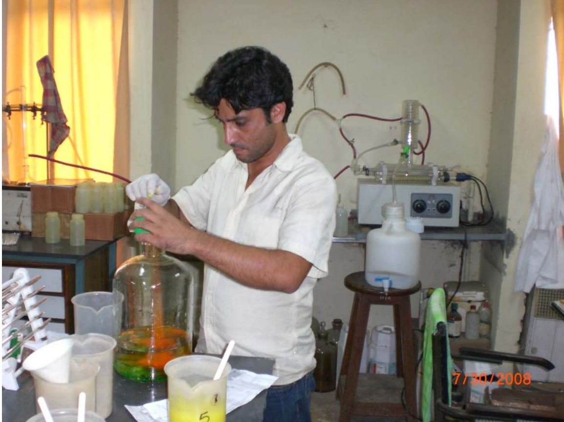
Figure 6. Dr. Khan preparing concentrated metal solution to spike filtered wastewater. Note the vibrant colors of the metals in solution, and potential as dyes.
