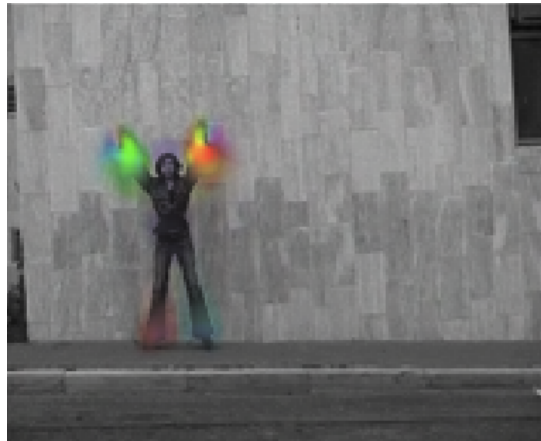
Figure 4.2: Example of a jumping-jack action in the human database, with optical flow field colorized [4] to indicate motion.
