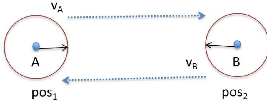
Figure 3-1 Robots A and B are moving with velocities v_A and v_B respectively. A and B are swapping positions. Conclusively they are travelling with velocities that would result in collision between the two robots
