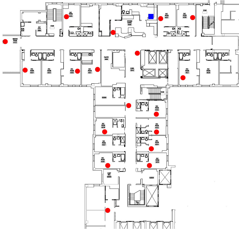
Figure 6.2: Deployment at Barnes-Jewish Hospitals. The blue square denotes the base station. Red circles denote relay nodes.
