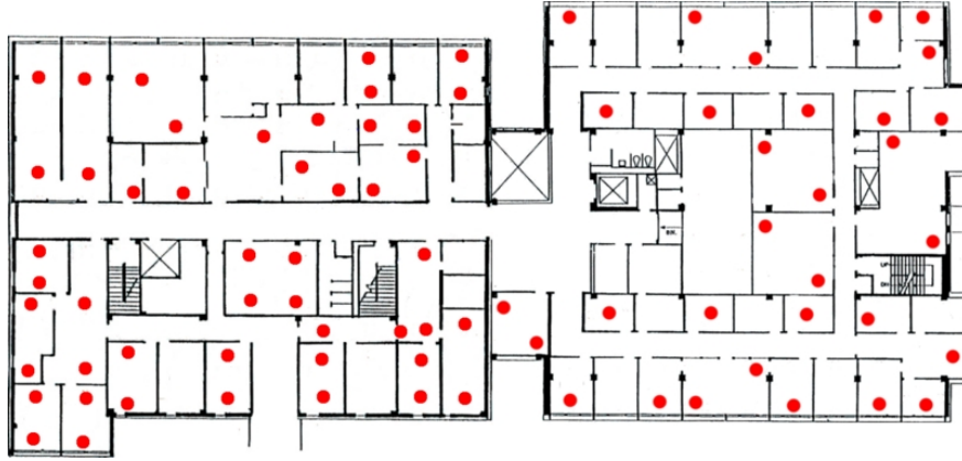
Figure 6.3: Deployment of the field devices on the fifth floor of Bryan Hall and Jolley Hall at Washington University in St. Louis.
