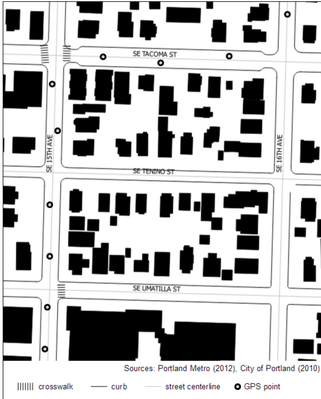
Figure 7 Pedestrian crossing rules: GPS points could not reliably determine side of street. The walk trip beginning at lower left above would have been assumed to use the crosswalk at SE Umatilla St. (by rule 1, see text) and a crosswalk at SE 15th Ave. and SE Tacoma St. (by rule 2).
