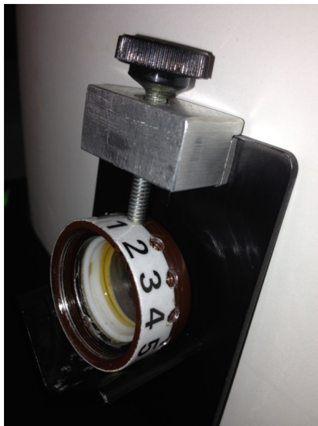
Figure 5.3 Sample holder assembly used for the preparation and measurement of the protein films. Films were coated onto sapphire windows held within a metal lens tube. The lens tube was placed on a V-shaped holder attached to a standard slide-mount sampling accessory for use in placing the sample into the spectrometer. A retaining screw was used to secure the rotational position of the lens tube in the sample holder. Fourteen labeled positions allowed reproducible placement of the films on the holder.
